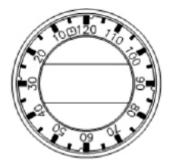
The cookers have an acoustic timer that can signal a maximum time of 120 minutes. Turn the knob to the right, place it on the preset time, between 0 and 120 minutes (see picture);
